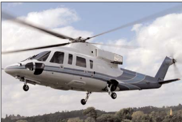
External tail rotor design can worsen higher frequencies
